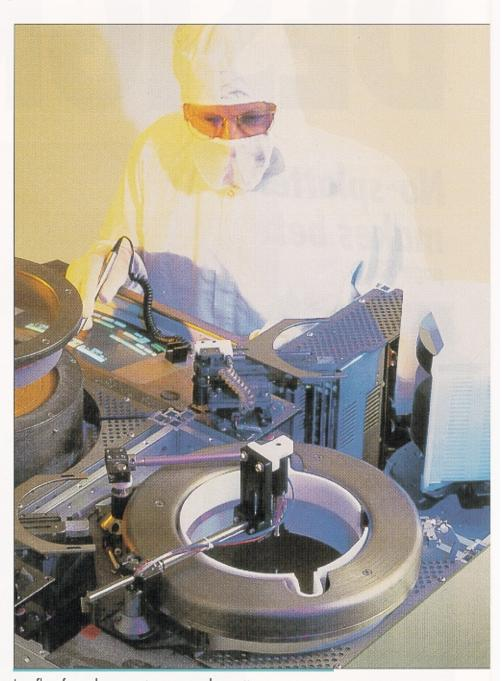
Low-flow, focused spray systems can produce patterns as narrow as 0.070 in., and deliver single-shot sizes of only a few hundred nanoliters or continuous flow rates as low as a few microliters/min. The nozzle assembly can mount on a robotic arm, as in this application, or on an X-Y table to execute continuous patterns. Alternatively, it can also mount in a fixed position to dispense a precise amount of spray at a selected site.
