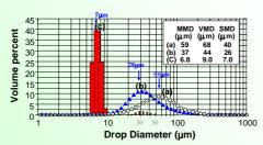
Drop size distribution (b) is much narrower (half width 40μm versus 70μm) than (a)
