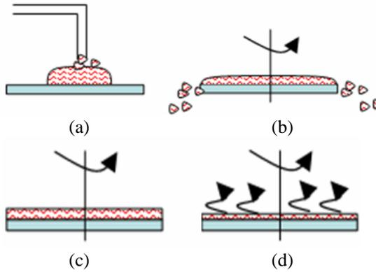
**Figure 1** The schematic view of spin coating process, (a) Dispensing, (b) Spin-up, (c) Spin-off, and (d) Evaporate.
