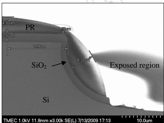
Figure 6 SEM image of a PR film coated by using SS method after developed.
