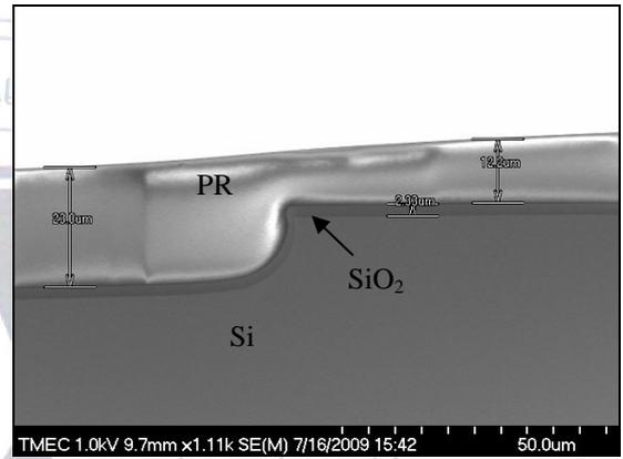
Figure 8 SEM image of a PR film coated by using MS method before exposed.
