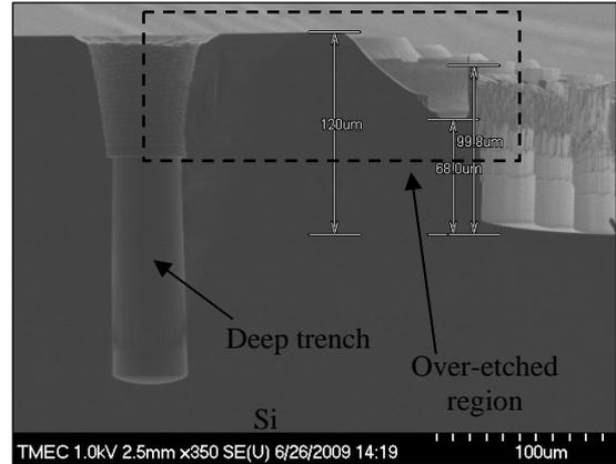
Figure 7 SEM image of a PR film coated by using SS method after etched.
