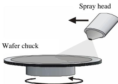
**Figure 2** The schematic view of spray coating process.
