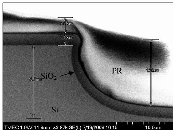
Figure 5 SEM image of a PR film coated by using SS method before exposed.
