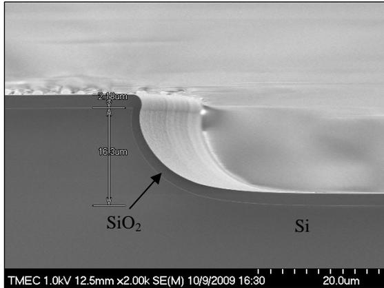
Figure 4 SEM image of SiO<sub>2</sub> film coated on Si substrate.
