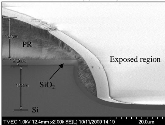
Figure 11 SEM image of a PR film coated by using SC after exposed.
