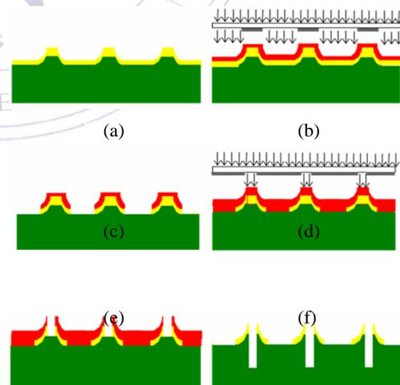
**Figure 3** Micro-needles fabrication process flow, (a) SiO<sub>2</sub> deposition, (b) Patterning#1, (c) SiO<sub>2</sub> etch, (d) Patterning#2, (e) Shallow trench etch, (f) Deep trench etch.
