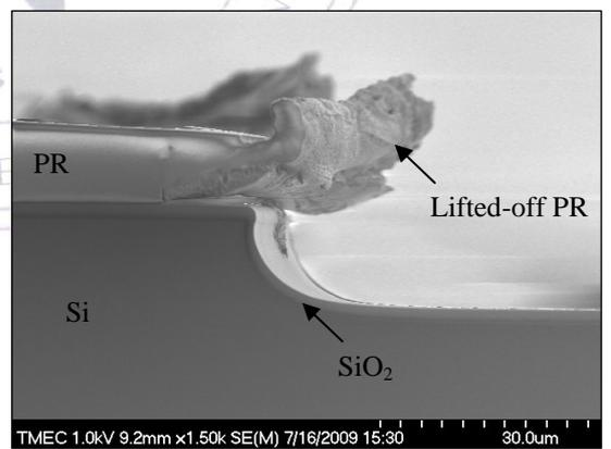
Figure 9 SEM image of a PR film coated by using MS method after developed.
