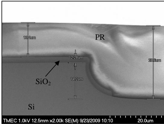
Figure 10 SEM image of a PR film coated by using SC before exposed.
